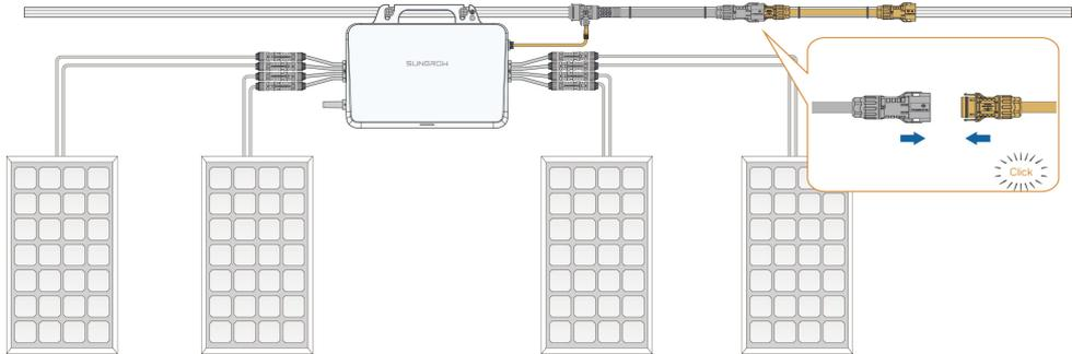
**Step 5** Connect the AC male connector. For instructions on how to attach the AC male connector to the cable, see "[4.3.2 Attach AC Male Connector](#)". Connect the AC male connector to the other side of the T-type AC trunk cable, as shown in the figure below. Make sure the connection is secure.
