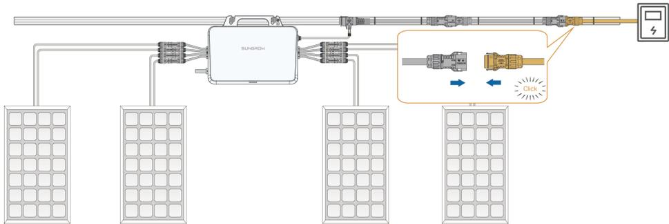
**Step 6** Seal off the T-type connector. If no cable is connected to the port on the other side of the T-type connector, seal it off with the sealing cap, as shown in the figure below.
