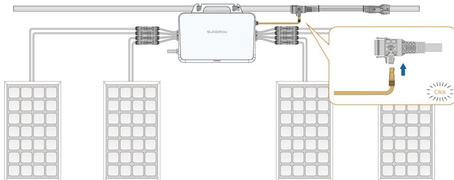
**Step 4** (Optional) Connect the extension cable. An extension cable is required if the distance exceeds 2.8m. Connect the T-type AC trunk cable to the other end of the extension cable, as shown in the figure below. Make sure the connection is secure.
