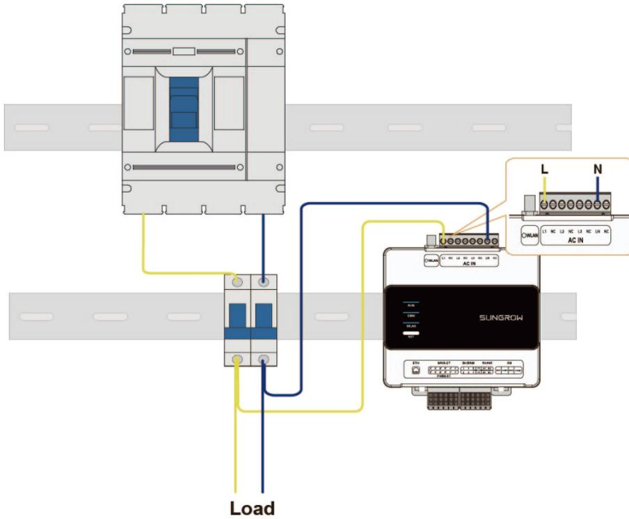
**Step 4** Connect the CT wires to the GRID.CT terminal, and clamp the CT to the AC cable with the arrow pointing in the direction of the load.
