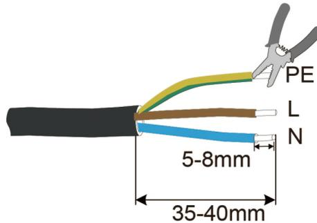
**Step 3** Crimp the terminals. Crimp the cold-pressed terminals onto the wires using a crimping tool.
