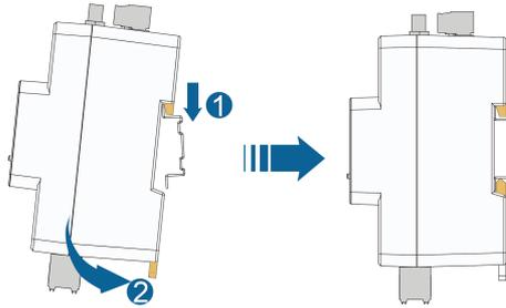
**Step 4** Push the bottom clips upward. Make sure the iHomeManager firmly fits on the guide rail.
