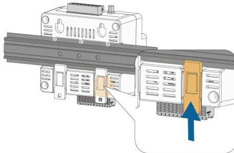
**Step 5** Install the end brackets on the guide rail at both sides of the iHomeManager to restrict it in a fixed position.
