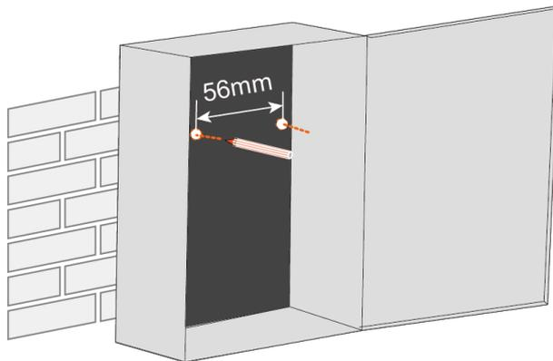
**Step 3** Drill holes at the marked positions using a hammer drill.
