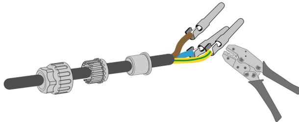
**Step 4** Wiring. Insert the L, N, and PE wires into the corresponding holes on the AC male connector, as shown in the figure below.
