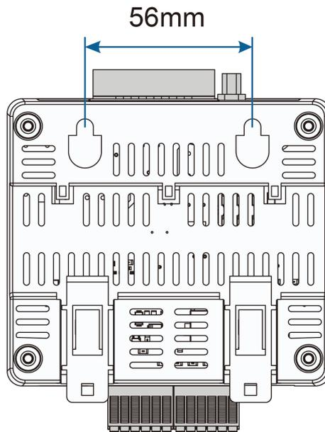
**figure 4-3** Mounting Holes
