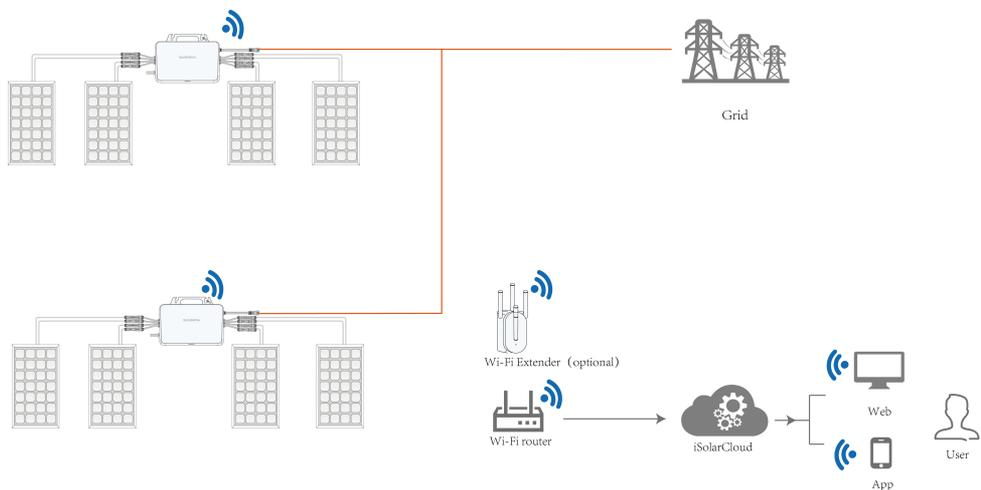
**figure 2-3** Networking Diagram of Rooftop PV System
