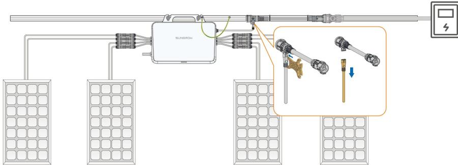
**Step 3** Remove the DC connector, use a connector wrench to loosen the locking parts.
