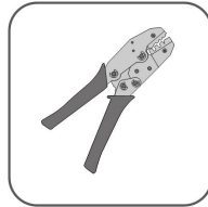
MC4 terminal crimping tool 4–6mm 2
