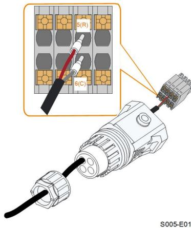
step 6 Insert the terminal plug into the **COM2** terminal at the bottom side of the inverter and then install the housing.
