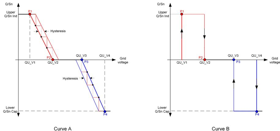
figure 7-19 Reactive Power Regulation Curve in Q(U) Curve
