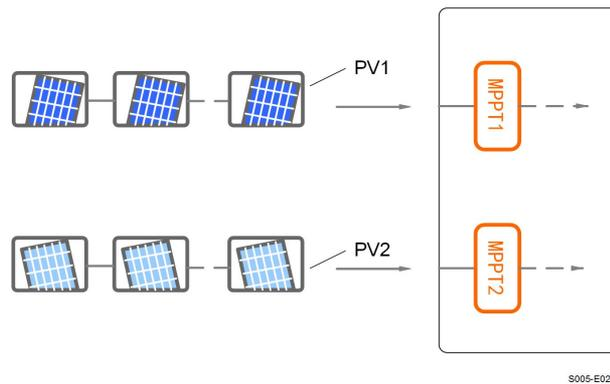
**figure 5-3** PV Input Configuration (SG6.0RS for example)
