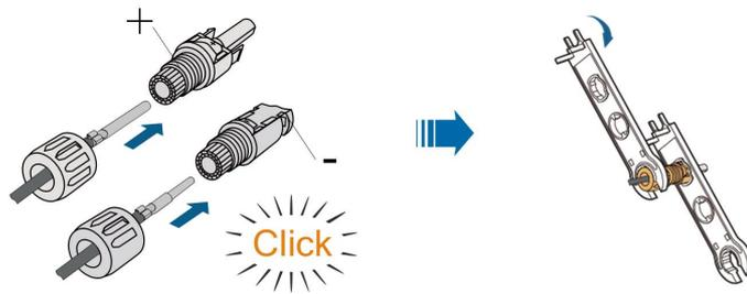
step 4 Check for polarity correctness.
