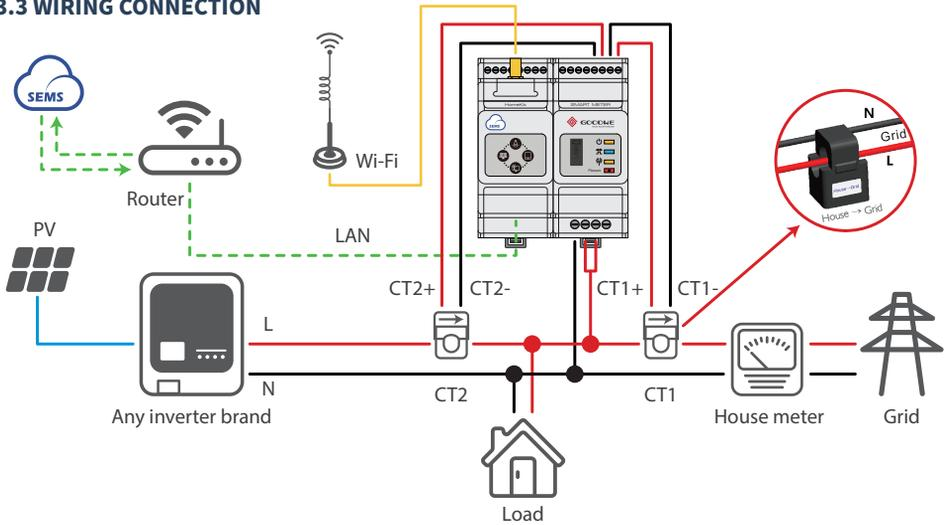
\* Please note the CT location: CT1 is connected to the Grid Point, while CT2 is connected to the Inverter Output Point, and the arrow direction on the CT is pointed to the Grid from the Inverter side. The connection wires of CT are RED corresponding to '+' and BLACK corresponding to '-'.
